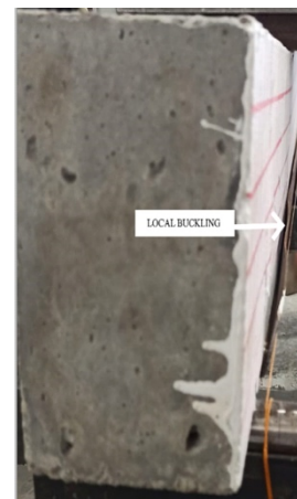
Figure 12. Flange buckling in RL beam.
